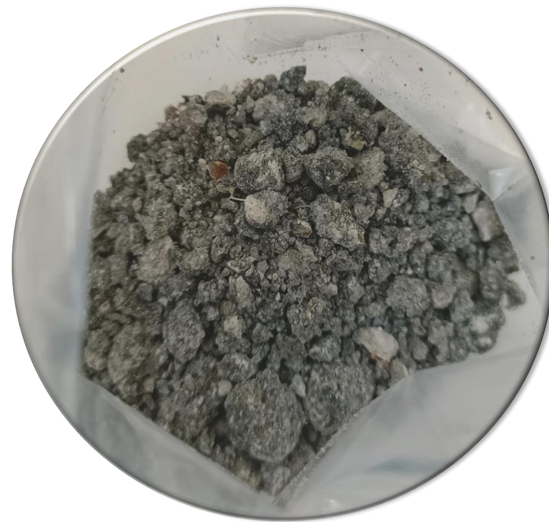
The black bentonite appears as a dark and moist mass after musts filtration and subsequent squeezing
