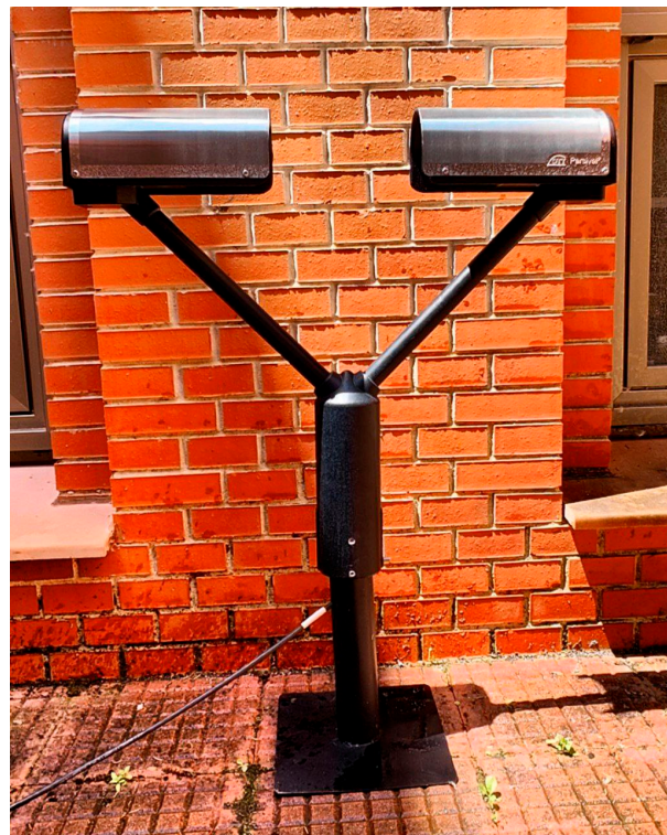
Figure 3. Parsivel 2 optical disdrometer (OTT Hydromet GmbH, Kempten, Germany).
