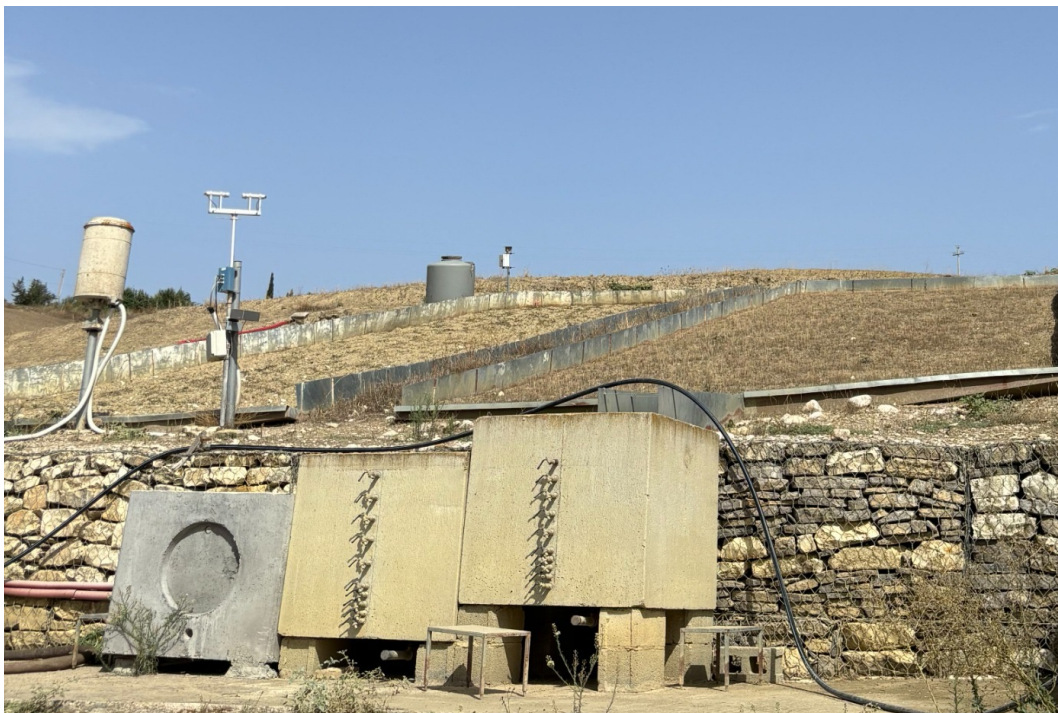
Figure 4. Sparacia experimental site: detail of the disdrometer installed downstream of the plots used for event-scale soil loss measurements.
