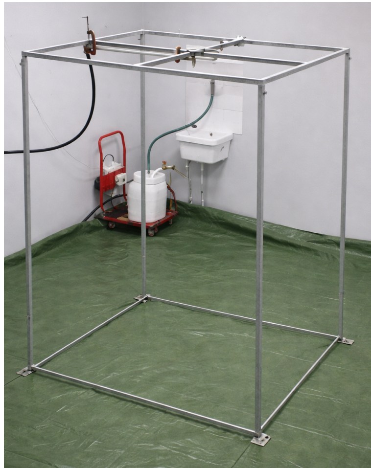
Figure 7. Support structure for the DRS and PRS systems at the Hydrology Laboratory of the University of Palermo.
