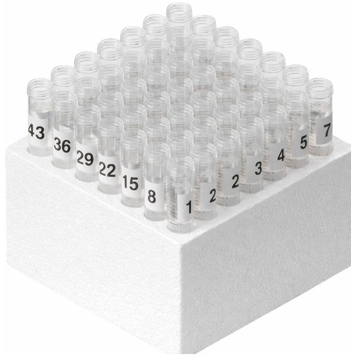
Figure 20. 3D representation of the collector system used to assess rainfall spatial uniformity across the 49 capillary tubes of the Kamphorst rainfall simulator.
