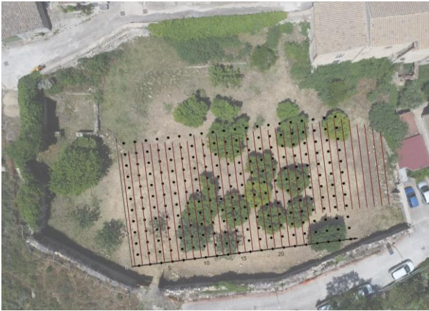
Fig. 1. Aerial view of the "Giardino dell'Annunziata, in Cammarata. The black points indicate the ERT electrode positions. The red lines indicate the GPR profiles.
