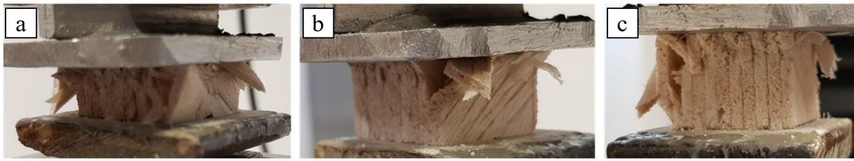
Figure 6. Typical fractures of core specimens tested in flatwise compression: (a) B(0), (b) B(±45), (c) B(±45/90).
