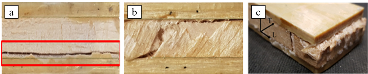
Figure 8. Shear failure of the sandwich core: (a) SB(0) 10 , (b) SB( \pm 45 ) 10 , and (c) SB( \pm 45/90 ) 10 .
