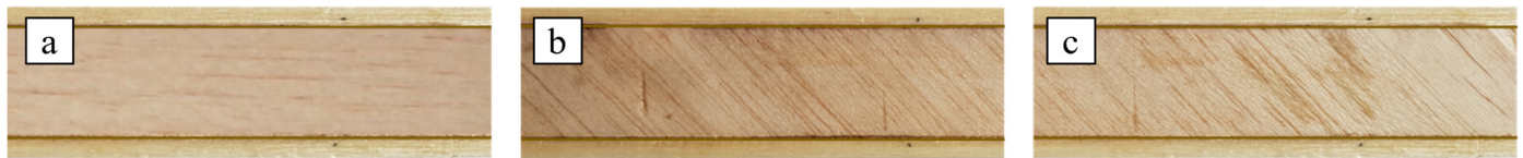
Figure 3. Sandwich samples manufactured in the laboratory: (a) SB(0), (b) SB( \pm 45 ), (c) SB( \pm 45/90 ).
