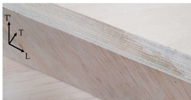
Figure 2. Innovative balsa laminate core type B( \pm 45/90 ).
