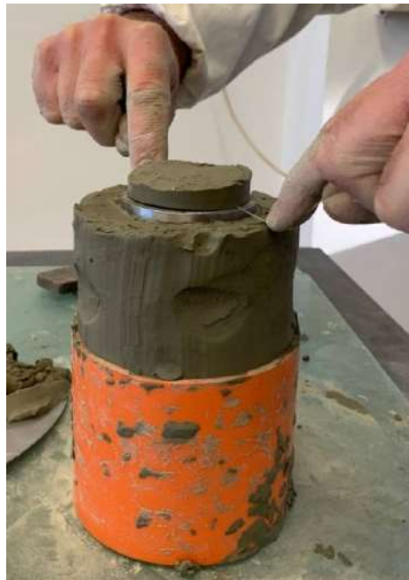
Figure 7.3 – Specimen preparation. Manual preparation of the soil adding distilled water (a); manual compaction of the soil (b); soil at the end of the manual compaction process (c); positioning of the PVC pipe (d); insertion of the PVC pipe in the soil (e); soil inside the PVC pipe (f); driving of the specimen (g); specimen refining by means of a nylon thread (h).
