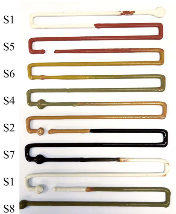
Figure 8.4 –Multimaterial serpentine. Errors on estimation of the tank-switching time.
