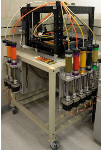
Figure 4.5 – Picture of the custom multimaterial 3D printer for soils developed by the GeoSI Group at the University of Los Andes.
