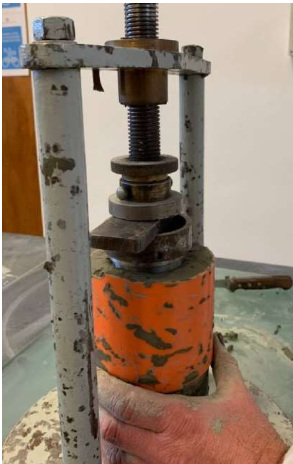
Figure 7.3 – Specimen preparation. Manual preparation of the soil adding distilled water (a); manual compaction of the soil (b); soil at the end of the manual compaction process (c); positioning of the PVC pipe (d); insertion of the PVC pipe in the soil (e); soil inside the PVC pipe (f); driving of the specimen (g); specimen refining by means of a nylon thread (h).
