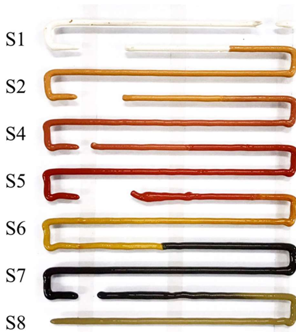
Figure 8.5 –Multimaterial serpentine. Underestimation of the tank-switching time.
