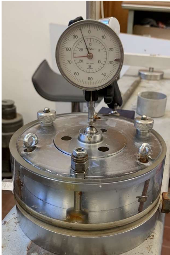
Figure 3.10 – Picture of the modified permeameter used to slightly compact the fine-grained soils.
