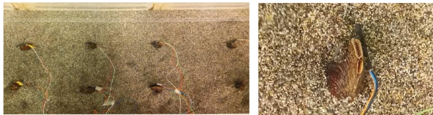
Fig. 2. Freshwater Mussels with Hall Sensors
