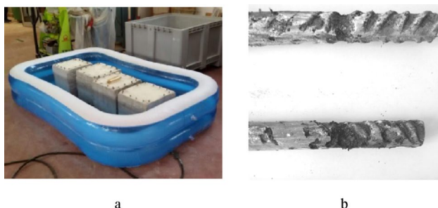
Fig. 6 Corrosion of reinforcement. a Specimens in the tank of water solution with sodium chloride; b pitting corrosion of reinforcing bars due to chloride attack
