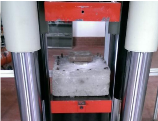
Fig. 9 Test set-up for compressive tests on pedestal
