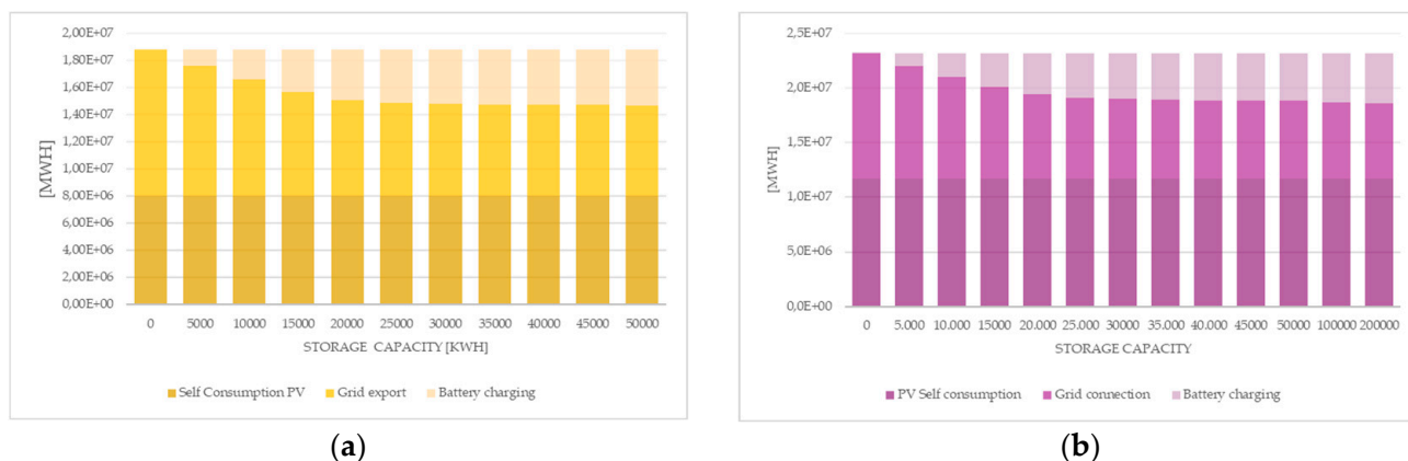
Figure 22. Management of the energy generated in the final scenario in Testaccio (a) and Valco San Paolo (b).
