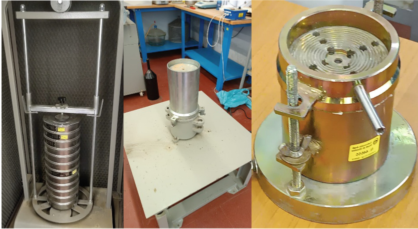
Fig. 1. Sieves for particle size analysis (on the left), maximum density equipment (in the middle), permeability test (on the right).
