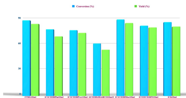
Fig. 1 Conversion and yield values for the methanolysis of BPA-PC, under US irradiation (50 W, 250 kHz) at 30 °C for 120 minutes, as a function of the nature of different catalysts ( n_c/n_{\text{RU}} = 1/12 ; m_{2\text{-MeTHF}}/m_{\text{MeOH}} = 3 ). Conversion and yield values were reproducible within \pm 3\% . Values for [\text{Ch}][\text{Im}] are taken from ref. 33.
