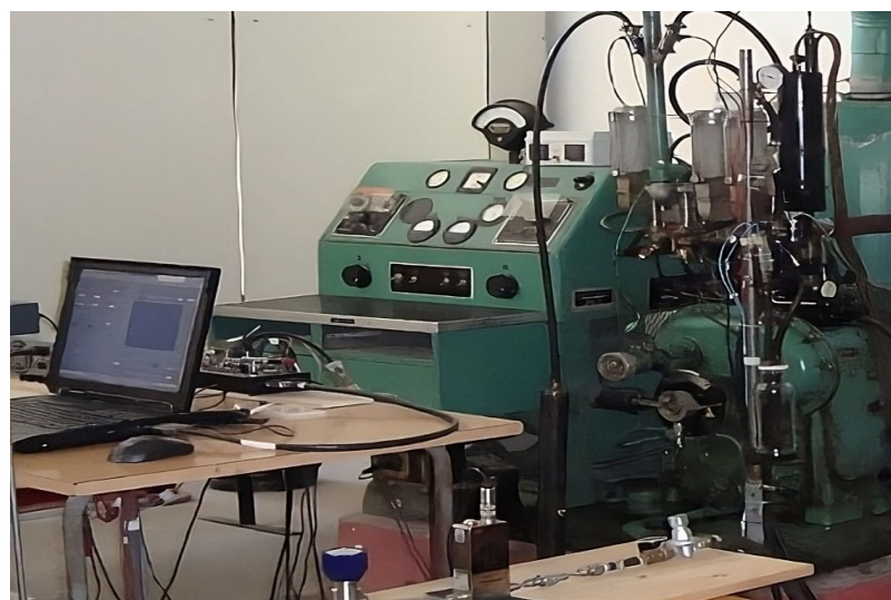
Figure 2. A picture of the CFR engine used in the test (the double-injection system is visible in the intake duct).
