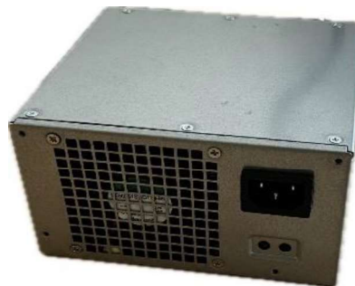
Figure 1. Power supply unit
