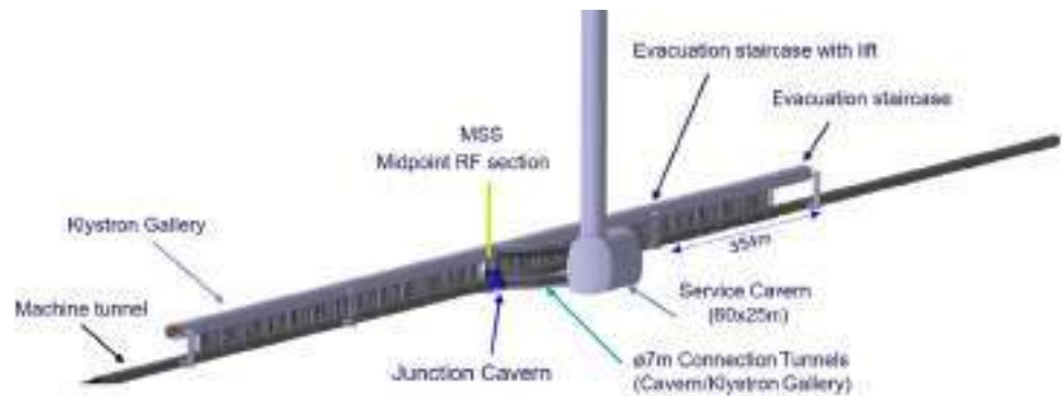
(b) Point PL - 354 m in between staircases
