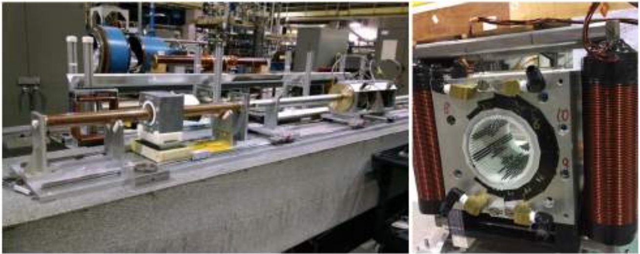
Fig. 10.24 Left: Performing rotating coil magnetic field quality measurements on an unshimmed Halbach magnet. Right: Shimmed Halbach magnet. Note the iron shimming rods of varying lengths (black) that have been assembled and glued to the plastic collar (white)
