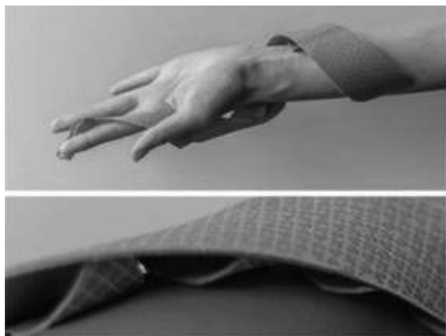
Figure 3. A prototype of the personalized 4D- printed adaptive wearable (top). A close-up of the many bioinspired tensioning mechanisms (bottom). (Image © Tiffany Cheng, ICD University of Stuttgart)
