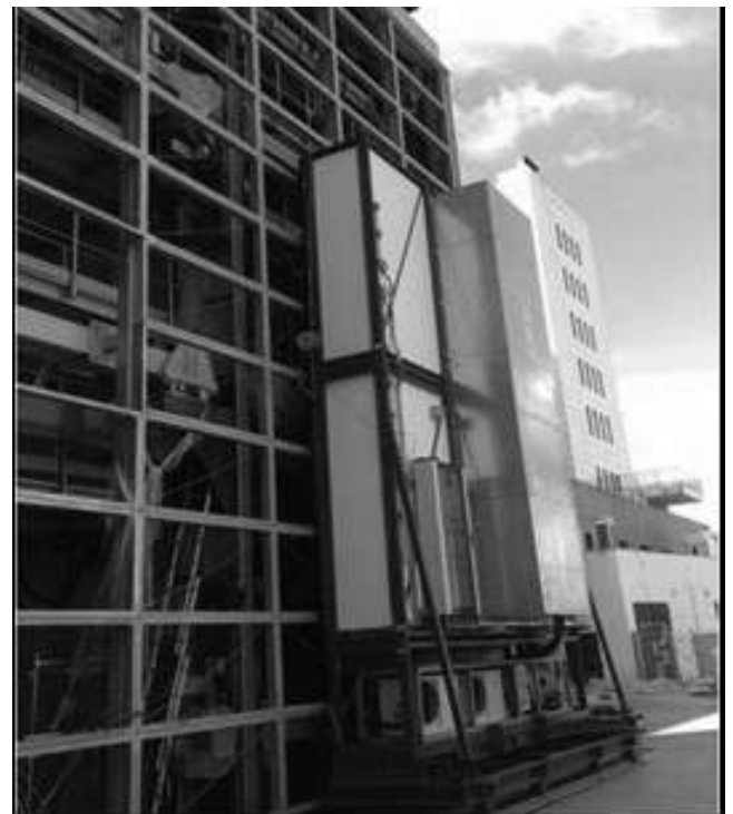
Figure 3. Fan capable of generating wind speeds equal to ~ 200 Km/h in accordance to the standard AAMA 501.1-05 “Standard Test Method For Water Penetration Of Windows, Curtain Walls And Doors Using Dynamic Pressure”, and all the other test with wind speed
