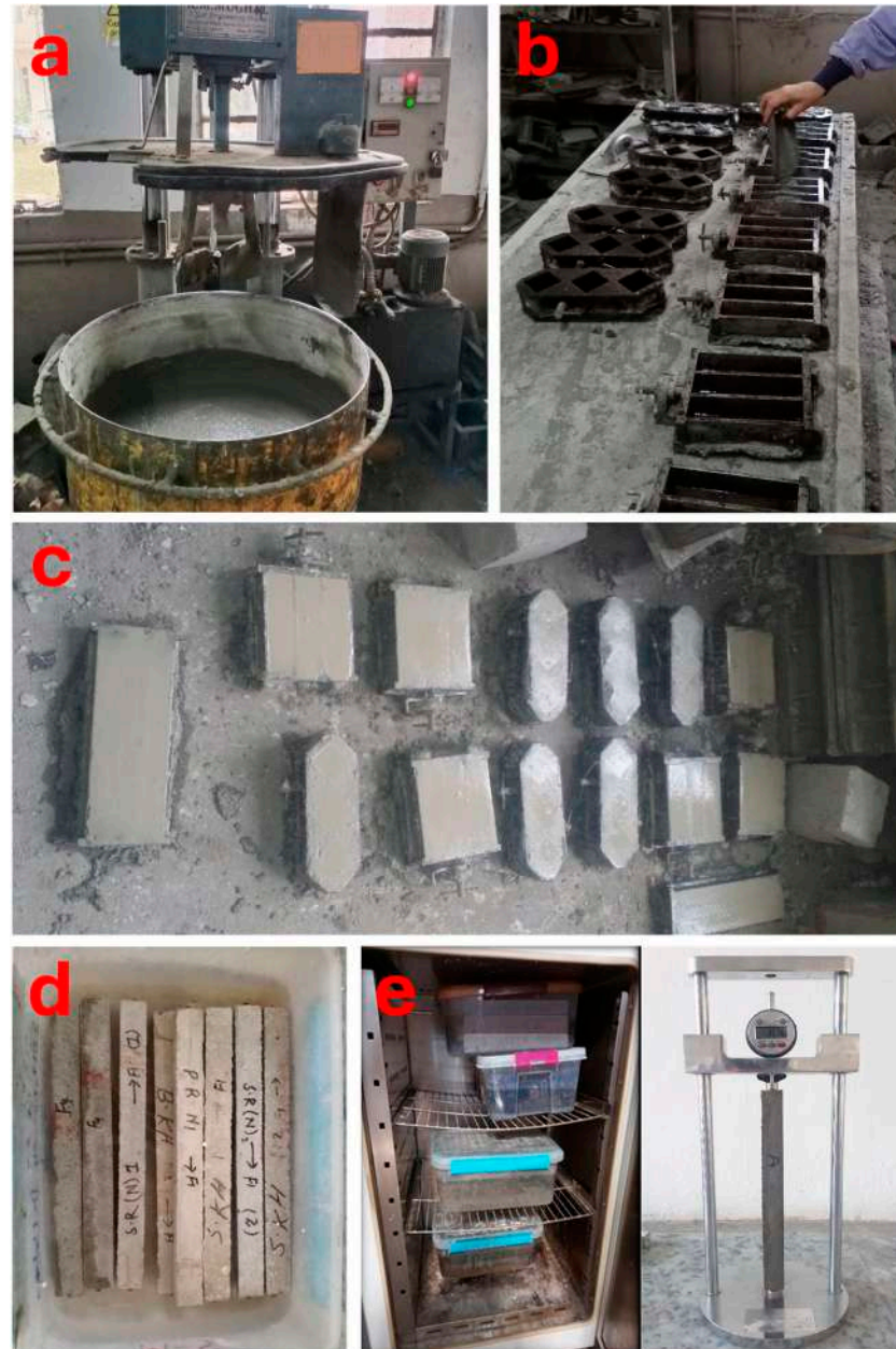
Figure 1. Preparation and evaluation of specimens: (a) electric mixer; (b) molds on vibrating table; (c) cast samples; (d) samples in ASR solution; (e) samples inside oven and tested with digital length comparator.
