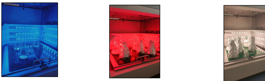
Figure 20. Photographic representation of the chemical synthesis of ZnO with blue light (left), red light (center), and white light (left) in the incubator including an adapted LED system.
