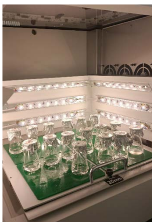
Figure 21. Photography of the apparatus for biological synthesis of ZnO with light in the incubator including an adapted LED system.
