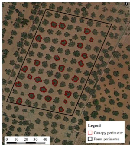
Figure 4.2: Example of plot with 25% of canopy surface vectorised, used for calibration of predictive relationship f_c -NDVI.
