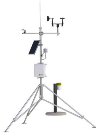
Figure 2.17: Standard weather station for the measure of climate variables ( https://www.campbellsci.de/wxpro ).
