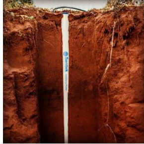
Figure 2.8: Sentek™ “Drill & Drop” probe to measure soil water content and temperature ( https://sentektechnologies.com/products/soil-data-probes/ ).
