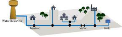
Fig.2: Schematic illustration of the principal elements of a WDS [7].
