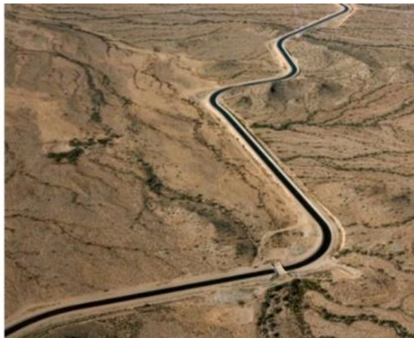
Figure 1.1 - Central Arizona Project (CAP): an example of well-bounded open channel. The aqueduct is a diversion canal in Arizona (US) diverting water from the Colorado River (U.S. Bureau of Reclamation).
