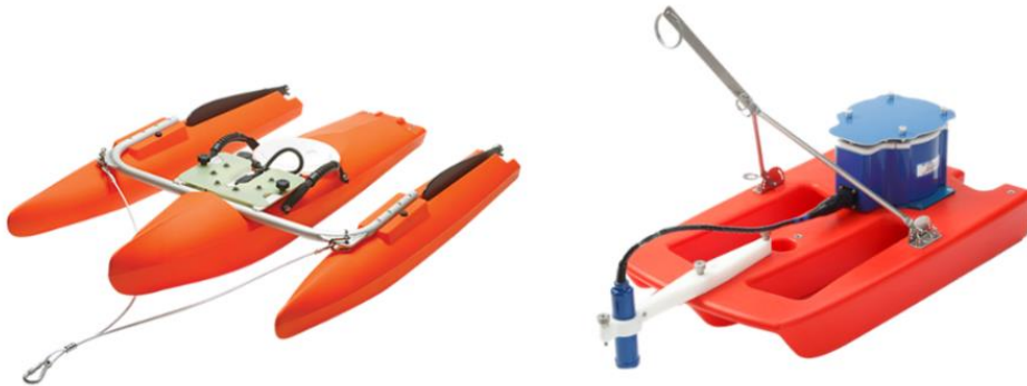
Figure 1.101 – Tethered ADCP boats. (Communication Technology srl)
