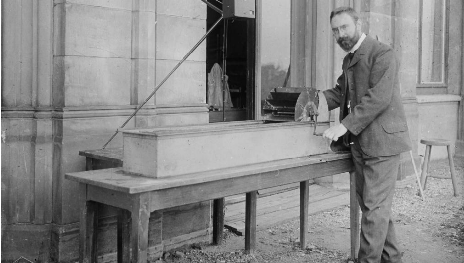
Figure 2.2 – Prandtl in 1904 running his open channel model through the paddle wheel. (DLR School Lab)
