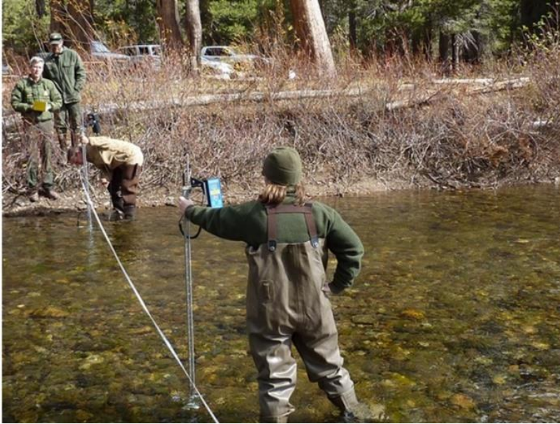
Figure II – Typical river discharge measurement with a current meter (National Park Service U.S. Department of the Interior)
