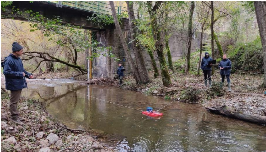
Figure 3.1 – Measurement activities moving ADCP along a transect.
