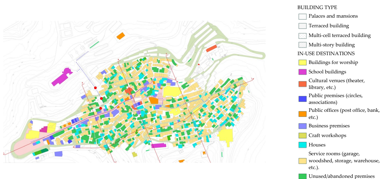
Figure 2. Building types and ground floor uses (Image prepared by Arch. P. Di Bella).
