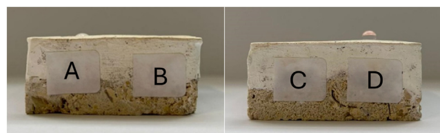
Fig. 2. Test of wettability consolidant systems. A=Ba(OH) 2 in 75% water, 25% isopropanol; B=Ba(OH) 2 in 75% isopropanol, 25% water; C=nanolime; D= nanosilica.
