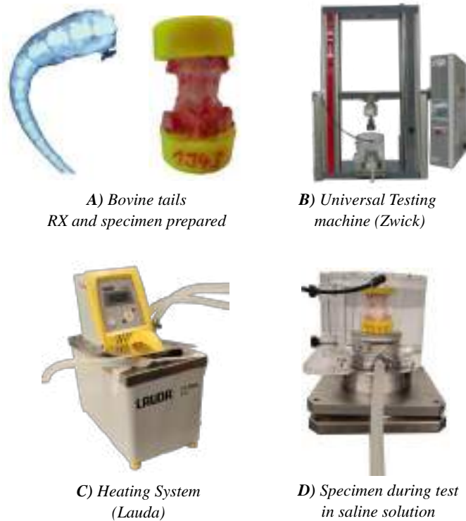
Figure 4.11. © Materials and method: A) X-Ray Bovine tail and specimen prepared; B) Universal testing machine; C) Heating machine; D) Specimen fixed in saline solution.
