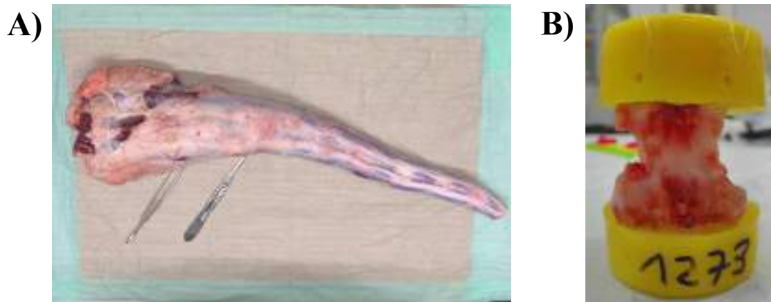
Figure 2.13. © A) Fresh bovine tail; B) C3Y-4 Bovine tail embedded and prepared for testing.
