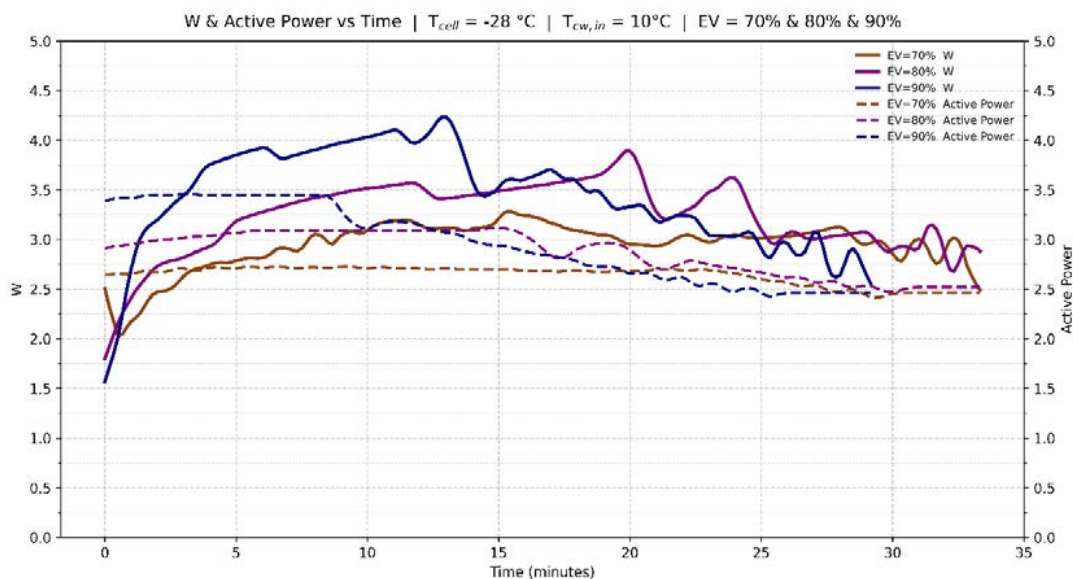
Figure 101 W and Active Power VS Time ( T_{cw,in} = 10\text{ }^{\circ}\text{C} / T_{cell} = -28\text{ }^{\circ}\text{C} )
