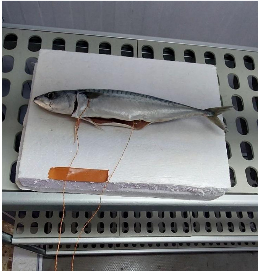
Figure 107 The Test Fish Along with its Temperature-Measuring Devices
