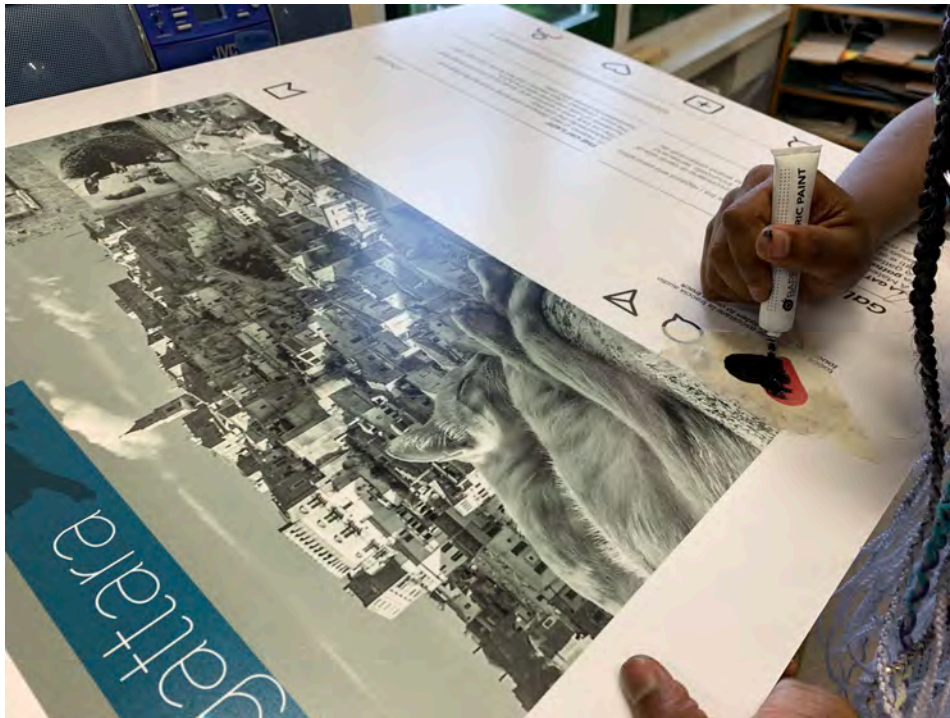
Figure 8 - Applying conductive ink and adding final touches
