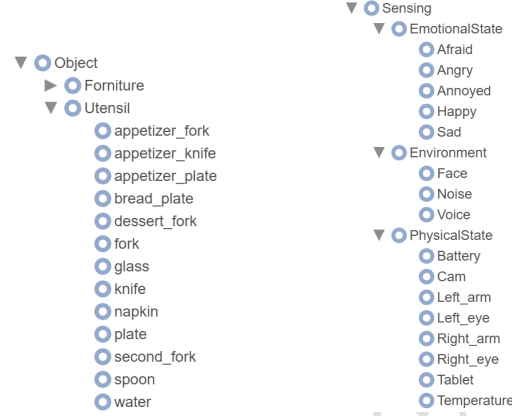
Figure 3: Excerpts of the ontology modelling a generic domain (table setup objects) and the inner world of the robot
