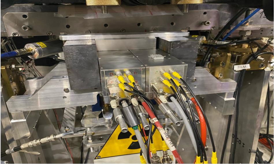
Fig. 3. Picture of the CZT detectors installed in DAΦNE.
