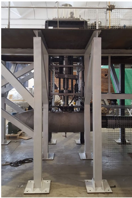
Fig. 6 Torque-applying device installed on the test bench
