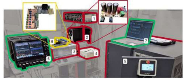
Fig. 6. Test bench: 1) Six DC sources; 2) 3P-5L-CHBMI; 3) LCL filter; 4) Grid connection switch; 5) Grid emulator; 6) Master and slave oscilloscopes; 7) PC with GUI; and 8) PED-Board with measurement shield.
