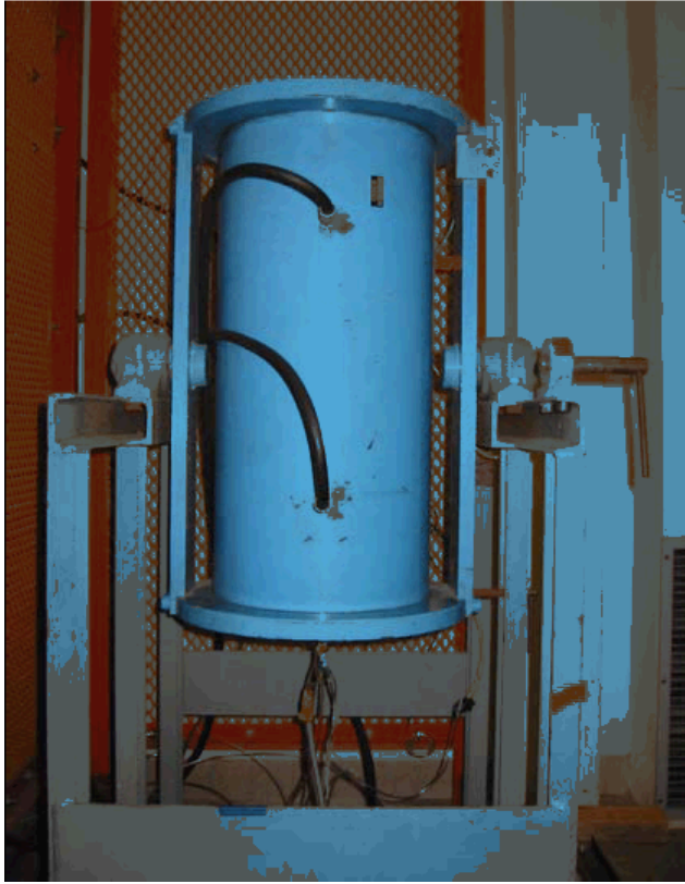
Fig. 8.2 Front vision of Internally Heated Pressure Vessel working vertically (Gros Bleu), equipped with a fast quench device. The two black rubber pipes ensure the water cooling of the furnace. Thermocouples exit wires, fast quench connections and electrical contacts are visible in the lower part of the vessel.
