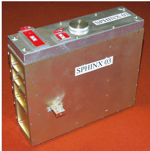
Figure 5 A photograph of the SphinX flight unit. The SphinX box sizes were 28 cm length, 27 cm height, and 8 cm width.
