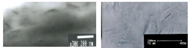
Figure 3 and Figure 4: TEM images of a) N6/MMTA2 and b) MMTA3
