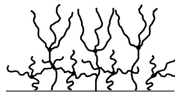
Figure 3. Schematic illustration of the occurrence of two populations of conformations of dendrons in a g=1 dendritic brush.
