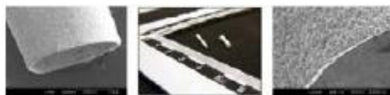
Figure 1 : Scanning Electron Microscopy (SEM) pictures of the tube made from PLA- b -PHEA copolymers
