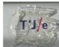
Figure 2. P(GI-co-CL) (30/70) obtained via thiol-ene cross-linking using UV radiation for 15 min
