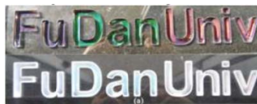
Figure 4. Intuitionistic comparison between the structural colors of CC films and peacock feathers. The CC films with carbon black (up) and without carbon black (down)
