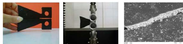
Fig 1. Samples for getting quantitative results on the self-healing functionality (a-b); healed crack faces closed by means of the metathesis product inside a crack after a (TDCB) test (c).
