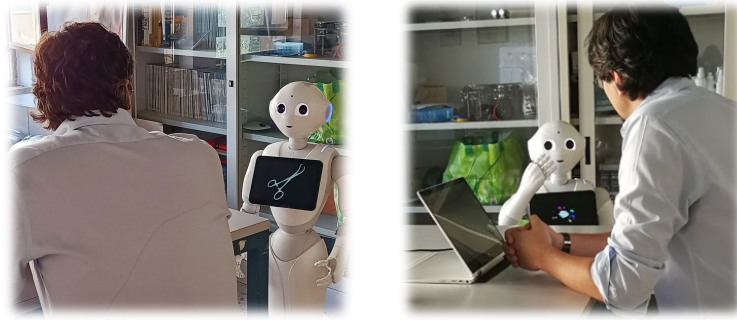
Figure 3.6: A photo related to the test session attended by the surgeon. The Pepper robot displays a tool, which the surgeon will then drag and drop onto the app interface to place it on the surgical table.
