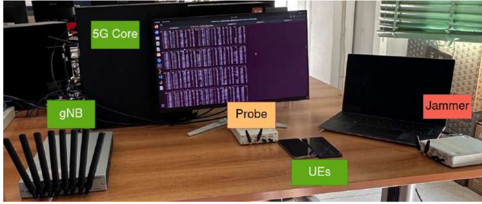
Figure 4.6: Experimental setup for 5G network implementation and testing. The 5G network components – Core Network, gNB, Pixel 6a, Samsung Galaxy S25 – are highlighted in green. The red box indicates the jammer used to perform ZP-CSI-RS attack. The yellow box marks the network probe, which is employed to monitor network performance and behavior during the experiments.
