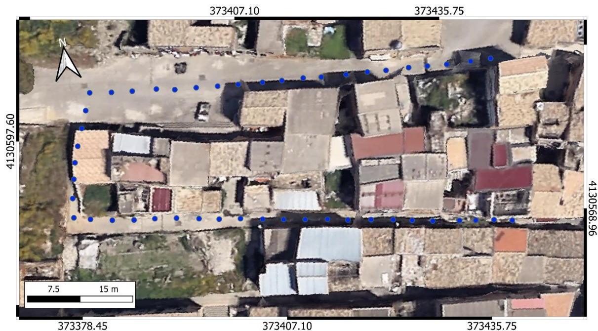
Figure 1: Map of the geophysical survey layout showing the C-shaped sensors alignment used for both ERT and SRT data acquisition. In blue dots, the position of the 48 receivers.
