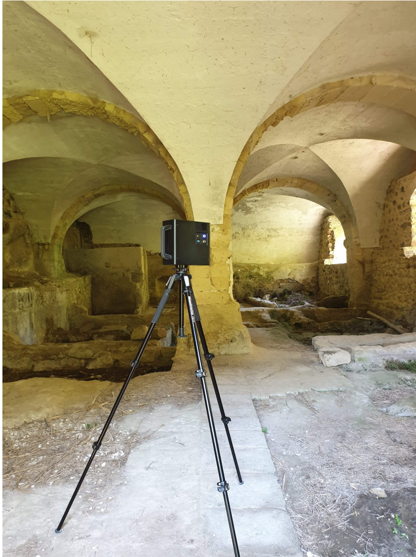
FIGURE 2.2: An example of Matterport camera in action
