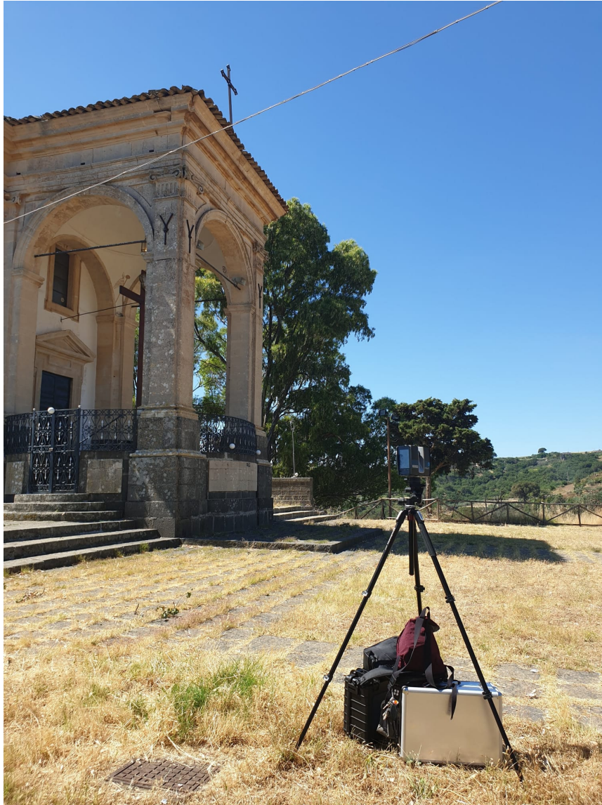
FIGURE 2.1: An example of static scanner installed on tripods
