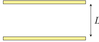
Figure 7.1: Scheme of a system of two metallic parallel plates, for which we measure the Casimir force per unit area. The controlled separation L is experimentally the metrological "lever arm". The z -axis is directed towards the high.
