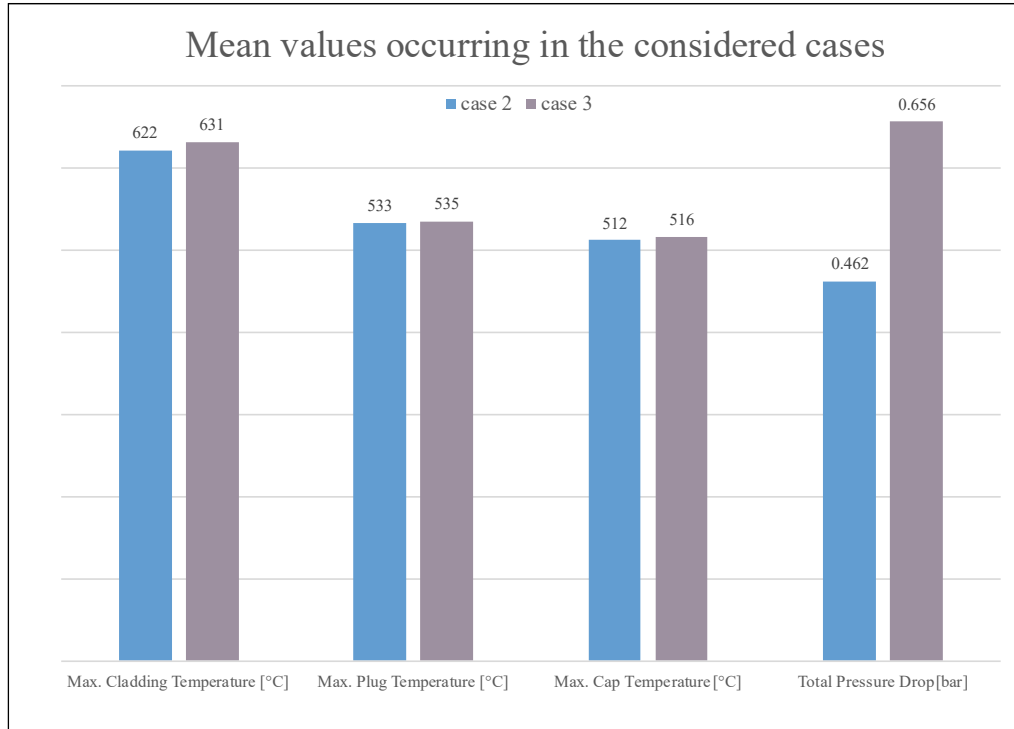
Figure 3.14: Comparison between case 2 and case 3 pin layout performance.
