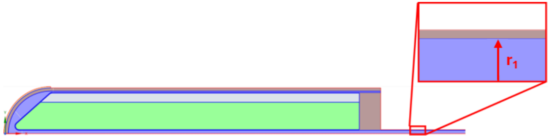
Figure 2.9: Inlet tube radius r_1 , shown in case 5 pin geometry.
