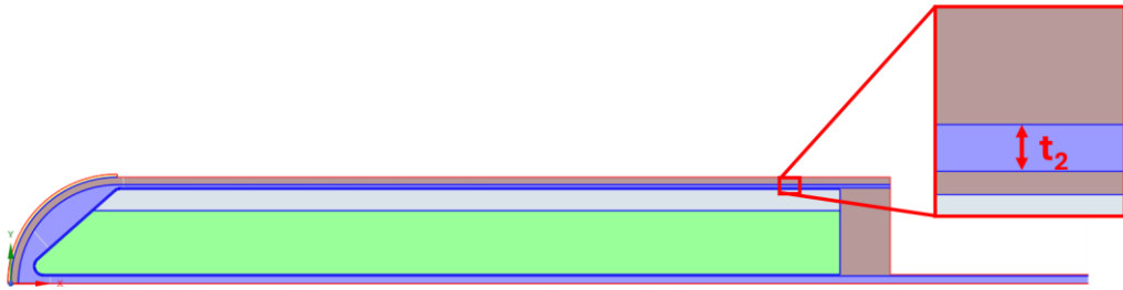
Figure 2.11: Outer annular channel thickness t_2 , shown in case 5 layout.
