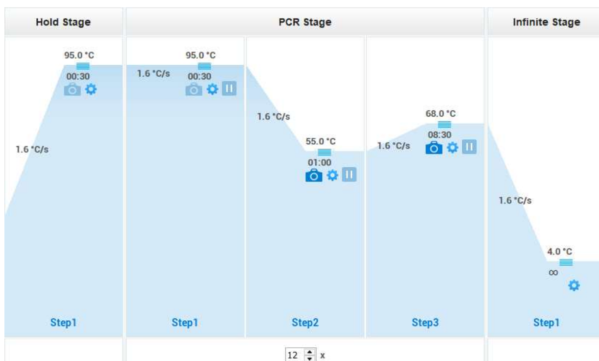
Scheme 3. Thermal profile: this profile was applied to introduce nonsense variants into the pRG213610 CHM WT -tGFP.
