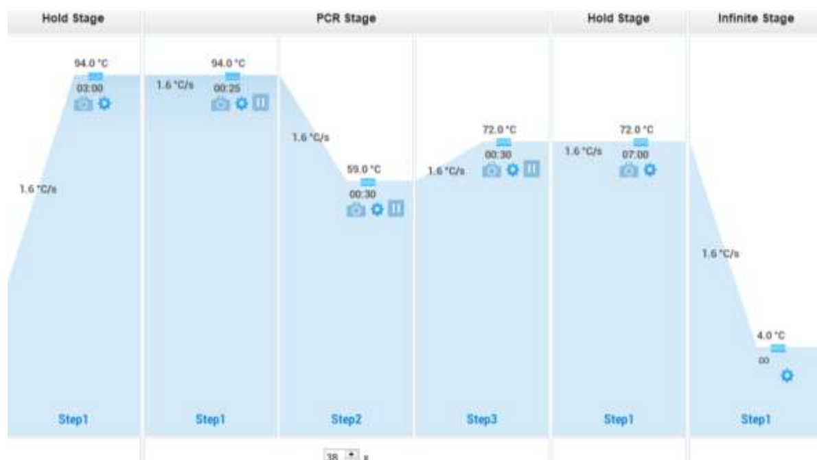
Scheme 1. Thermal profile adopted for genotyping analysis: the genotyping was performed by endpoint PCR with 2720 Thermal Cycler, in particular 38 cycles of amplification were performed (Applied Biosystems, Waltham, MA, USA).
