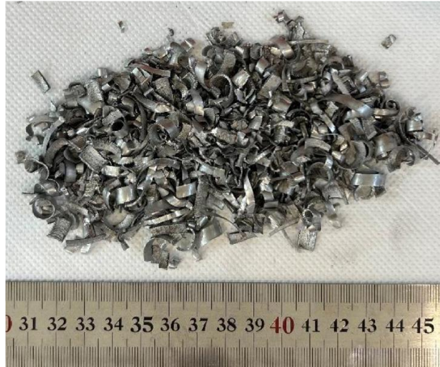
Figure 155. Shape and dimensions of metal chips used during the experimental campaign.
