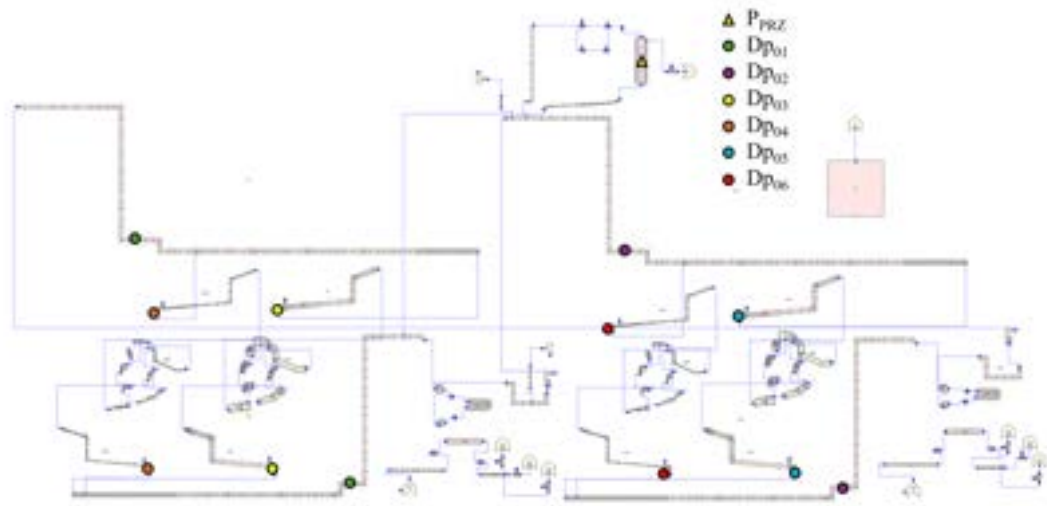
Figure 4.7: Signals location for the reactor trip.
