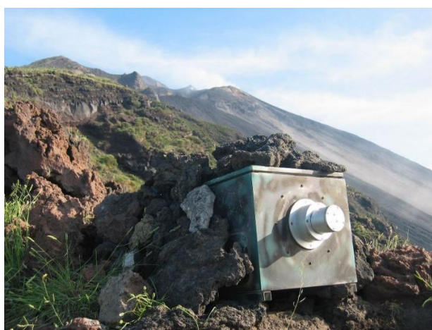
Figure 2.3 – UV scanning spectrometer used for remote sensing of volcanic gas emissions. The depicted instrument is part of a network of fixed scanning spectrometers designed to automatically retrieve \text{SO}_2 fluxes from volcanic plumes (photo from INGV newsletter ).
