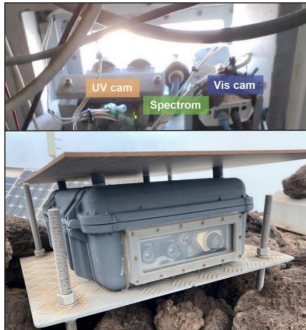
Figure 2.4 – Typical dual-band UV Camera configuration, coupled with an UV Spectrometer for calibration of images and a visible camera. The visible camera is useful to check the quality of the images and the environmental conditions.
