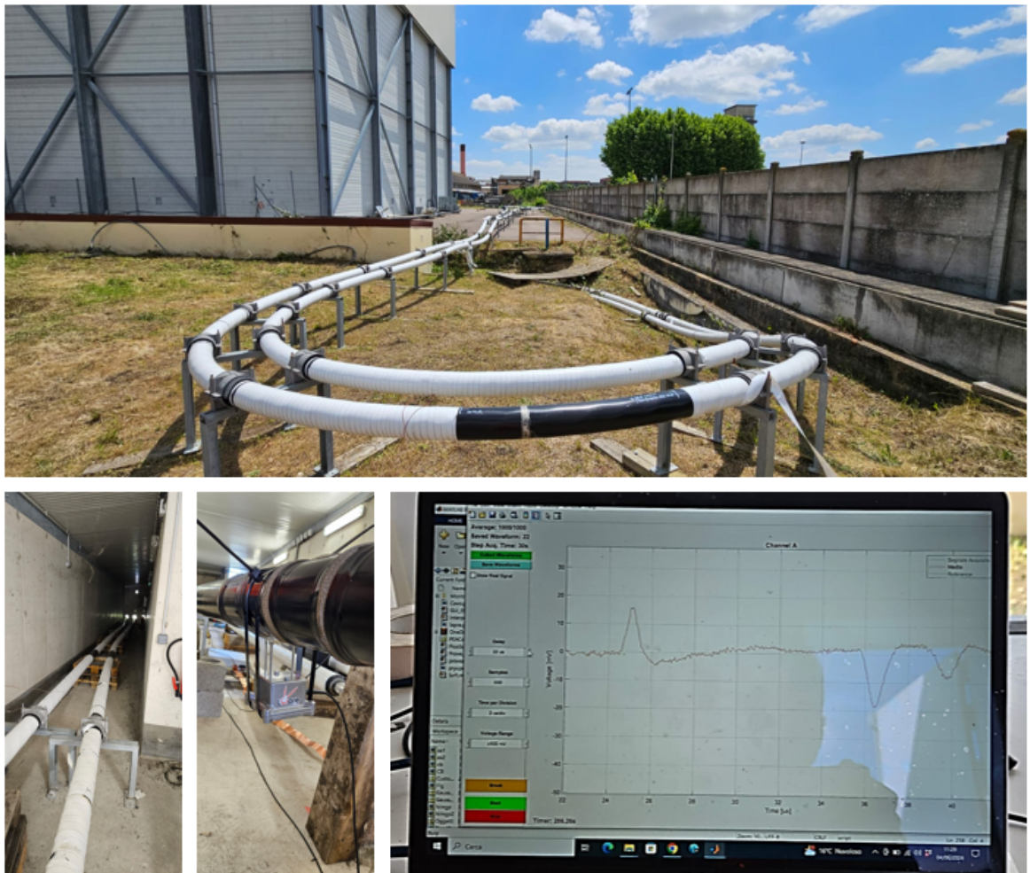
Figure 2.24: Hardware and software testing of the PEA setup for full-size cable. Measurement carried out at Prysmian High Voltage Lab, Montereau, France.
