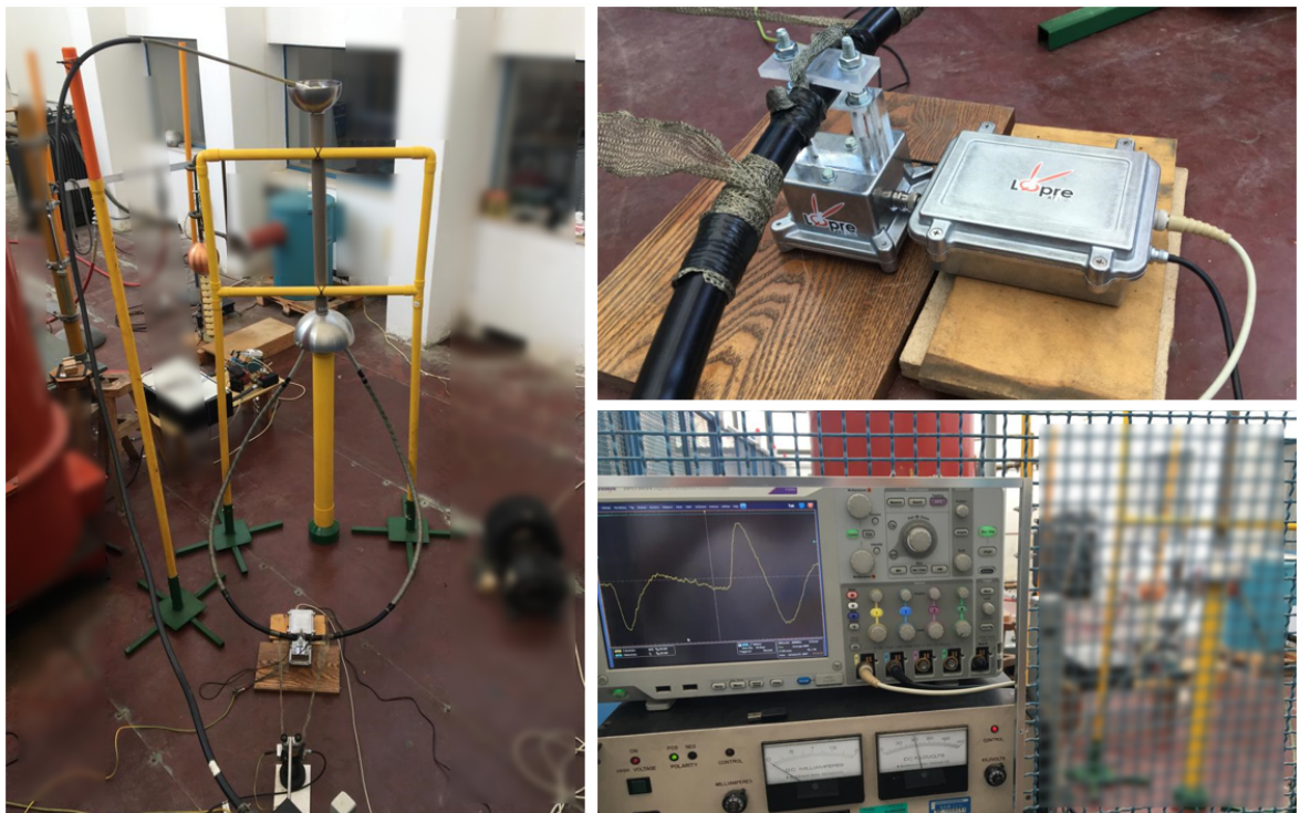
Figure 2.22: Hardware and software testing and validation of the PEA setup for mini cable. Measurement carried out at L.E.P.R.E. Lab, Palermo, Italy.
