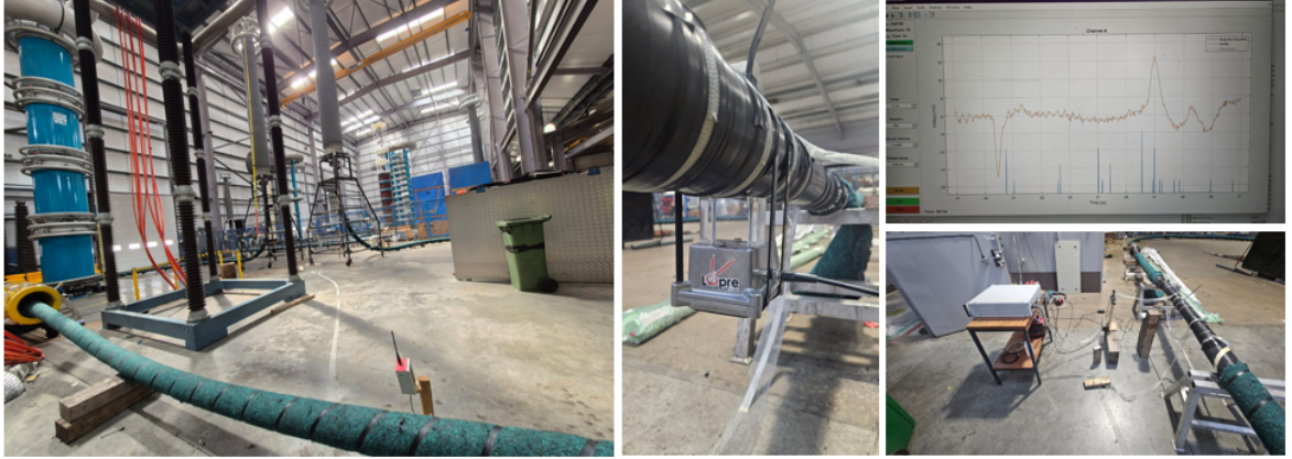
Figure 2.25: Hardware and software testing of the PEA setup for full-size cable. Measurement carried out at Prysmian High Voltage Lab, Bhisopstoke, United Kingdom.
