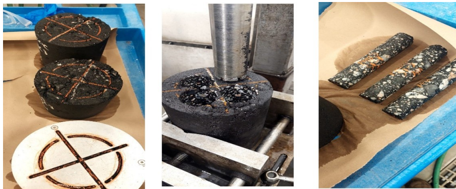
Coring and cutting of specimen
