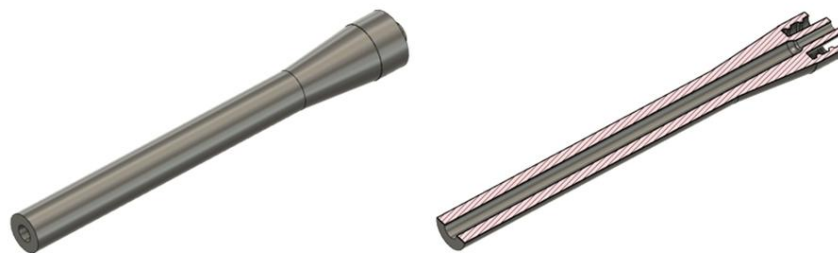
Figure 80: hollow rod design and cross section
