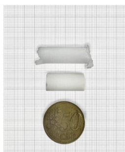
Figure 74: Scaffold dimensions respect to 50 cents coin.
