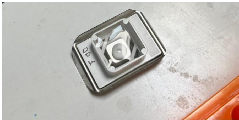
Figure 41: Scaffold sample embedded in OCT compound before cryostat sectioning. The sample was placed in cassettes and frozen at -80^{\circ}\text{C} for at least 4 hours to ensure structural preservation before slicing.
