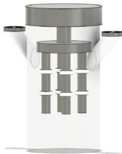
Figure 7: Spinner Flask bioreactor. Illustration courtesy of Sara Pecorella. Used with permission. Special thanks for the valuable contribution to this project
