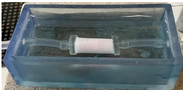
Figure 51: Scaffold inside the bioreactor immediately after nanoparticle perfusion tests. The pink coloration indicates the successful diffusion of gold nanoparticles into the porous matrix
