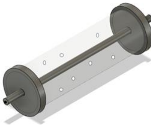
Figure 8: Rotating wall bioreactor. Illustration courtesy of Sara Pecorella. Used with permission. Special thanks for the valuable contribution to this project
