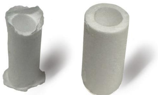
Figure 73: Scaffold Geometry before and after refining the circular bases
