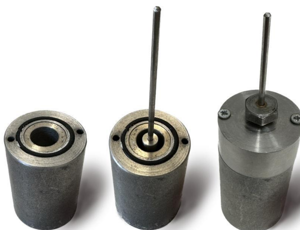
Figure 56: Mold setup for scaffold production. The polymer solution was poured into the mold, which was then sealed and subjected to a controlled thermal process to induce phase separation and scaffold formation.
