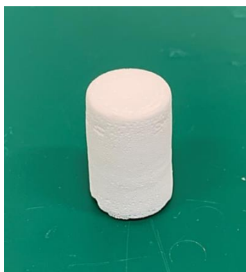
Figure 14: Cylindrical Scaffold obtained ant the end of TIPS protocol, 1,5 cm diameter 2,5 cm height
