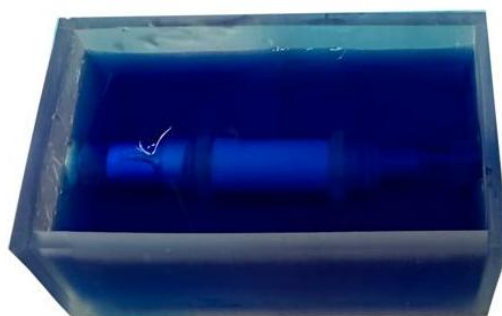
Figure 61: Scaffold placed in a toluidine blue solution for static diffusion tests. The experiment evaluates liquid penetration through the porous matrix under controlled conditions.
