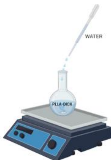
Figure 13: Solution preparation scheme: Water addition dropwise
