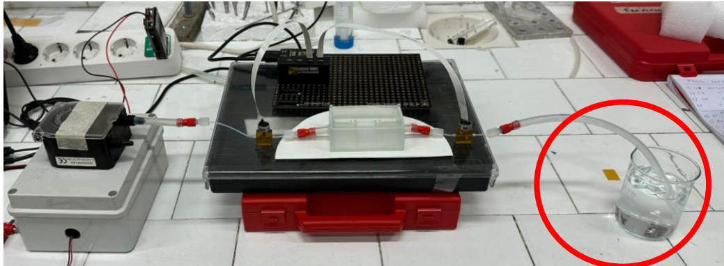
Figure 70: Bioreactor system assembled for airflow experiments. The design maintains an air-liquid interface, ensuring proper oxygenation while preventing liquid overflow, in red the 5 cm liquid head above the terminal
