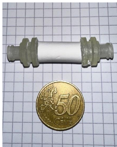
Figure 82: real dimensions of scaffold glued with connectors
