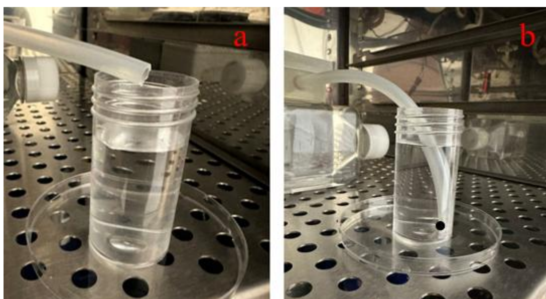
Figure 72: different experimental set up a) atmospheric pressure b) under 5 cm of H 2 O
