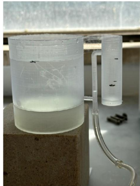
Figure 107: 3D printed system to evaluate liquid flow as a function of air flow inlet
