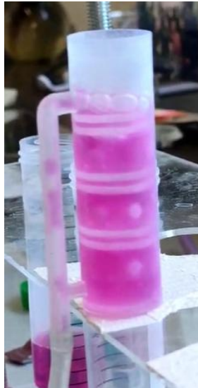
Figure 120: bioreactor and scaffolds set up for dynamic testing
