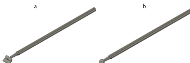
Figure 92: Cell Seeding Tools: (a) Cell Collection, (b) Seeding into the Lumen
