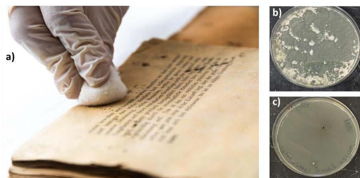
Figure 1: Old book attacked by biodeteriogens (a); growth of the microbial community before (b) and after (c) the irradiation treatment.
