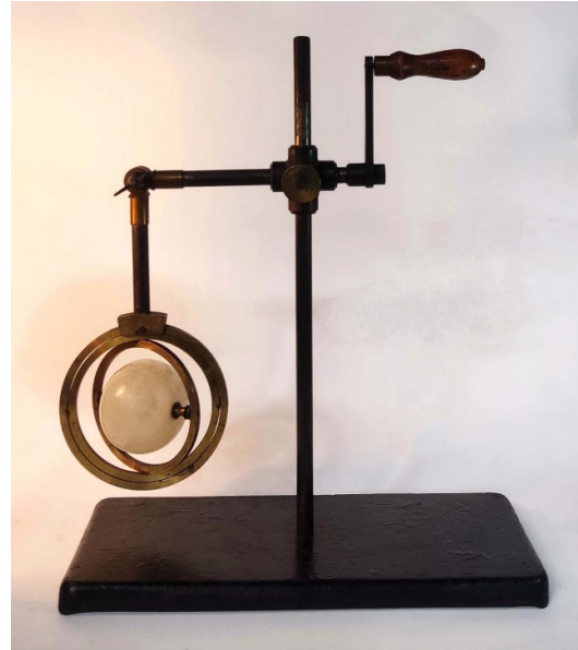
Figure 2. Bohnenberger’s apparatus of E. Sauerwald, Berlin, 1865. Historical Collection of Physics Instruments, University of Palermo.
