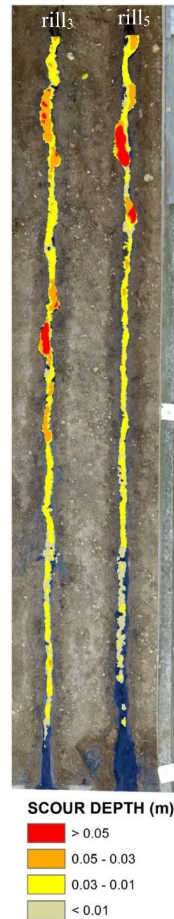
FIGURE 4 | DEM of difference (DoD) obtained for the rills with a biochar concentration of 3% (rill 3 ) and 5% (rill 5 ).
