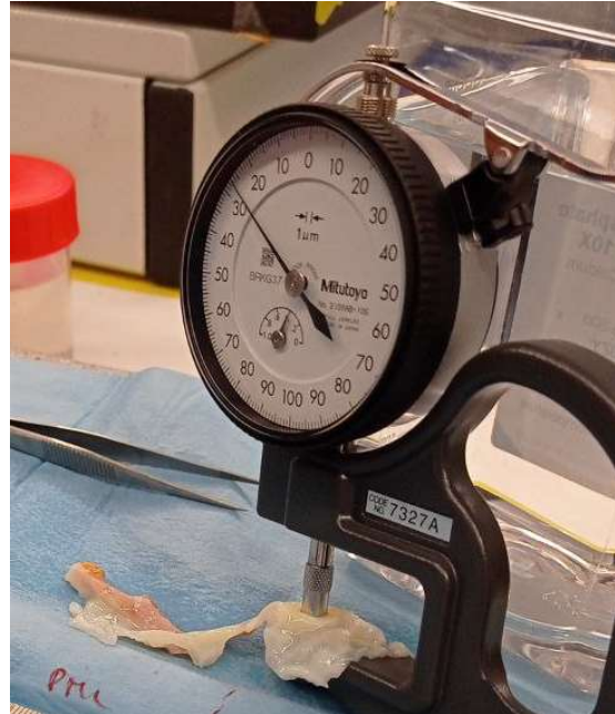
Figure 14. Dial gauge Mitutoyo used for leaflet thickness measurements
