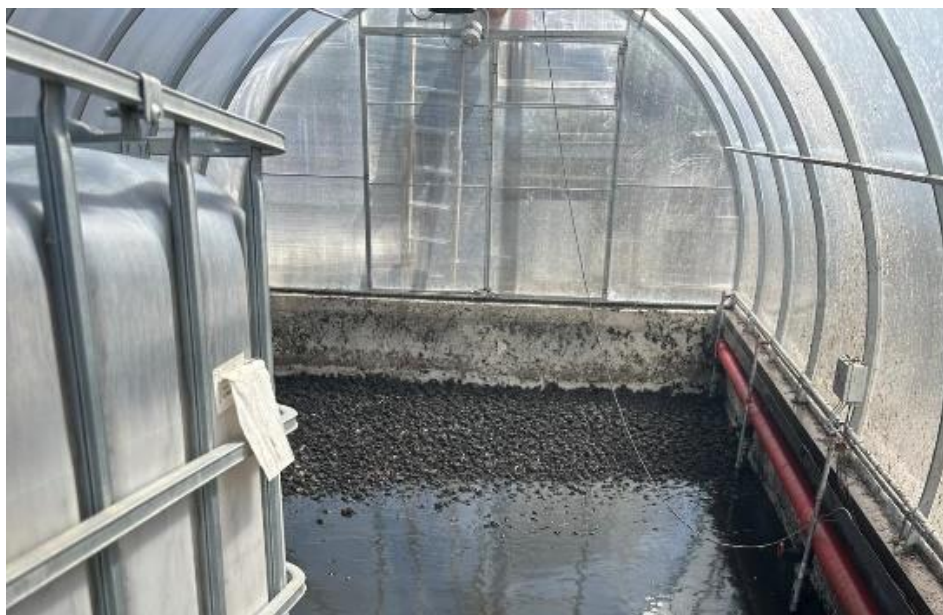
Figure 8.15 - 2° sludge load over the dried sludge of first load
