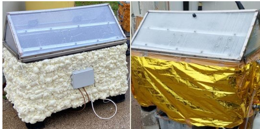
Figure 6.12 - Polyurethane foam coating and insulating blanket
