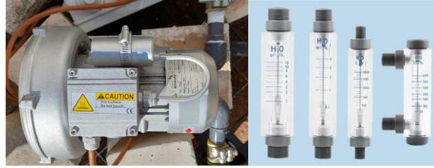
Figure 6.4 - (a) Blower, (b) Flow meters
