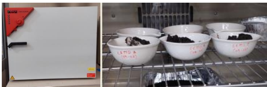
Figure 6.17 - 105°C Oven for sludge drying
