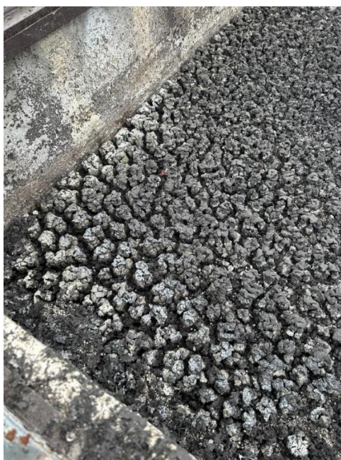
Figure 8.26- Detail of the dried sludge at the end of the experimentation period
