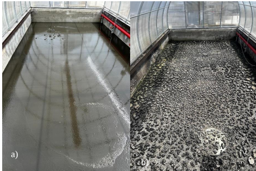
Figure 8.10 - Images of the sludge at the beginning and end of the test: a) at the beginning and b) at the end of the test
